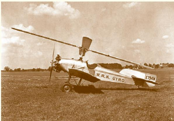
In 1931, E. Burke Wilford built the first successful autogyro to fly with a rigid rotor. It replaced the Cierva-type hinged rotors with a rigid rotor with cyclic pitch variation, based on the patents of Germans Walter Reiseler and Walter Kreiser – hence the designation, "W.R.K. Gyro." (Courtesy of the Smithsonian Institution National Air and Space Museum. Negative number 9A01102.)
