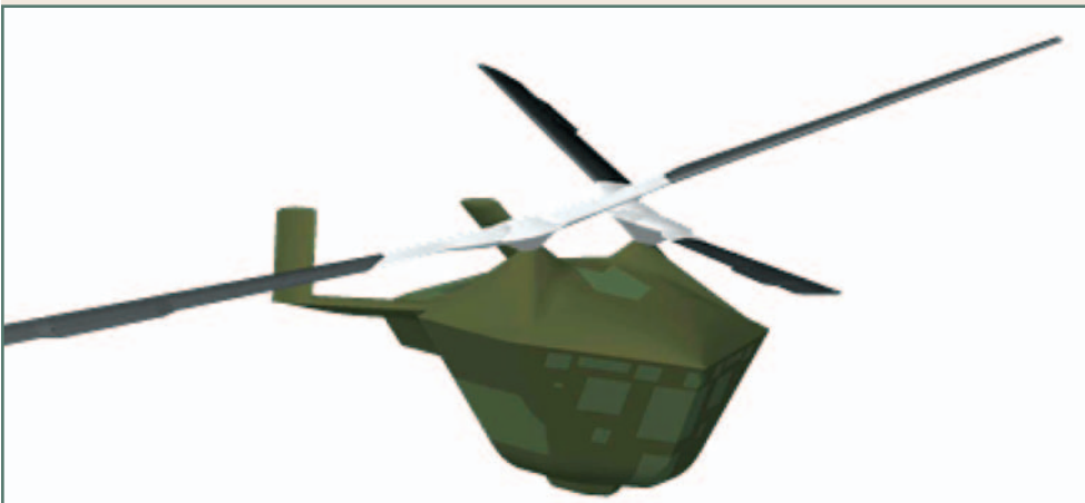
The Northrop Grumman UCAR concept uses a Kaman-inspired intermeshing rotor system with a refined rotor system for maximum lift and high cruising speed.
