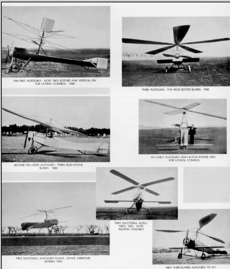
This set of pictures depicts the various autogiros that Juan de la Cierva tested in Getafe and Cuatro Vientos. On the lower left corner, the first successful autogiro flight is shown (17 January 1923). Source: Pitcairn-Cierva Company brochure.
