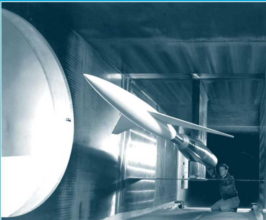
Testing advanced designs for high-speed aircraft, an engineer makes final calibrations to a model mounted in the 6 x 6 Foot Supersonic Wind Tunnel.
