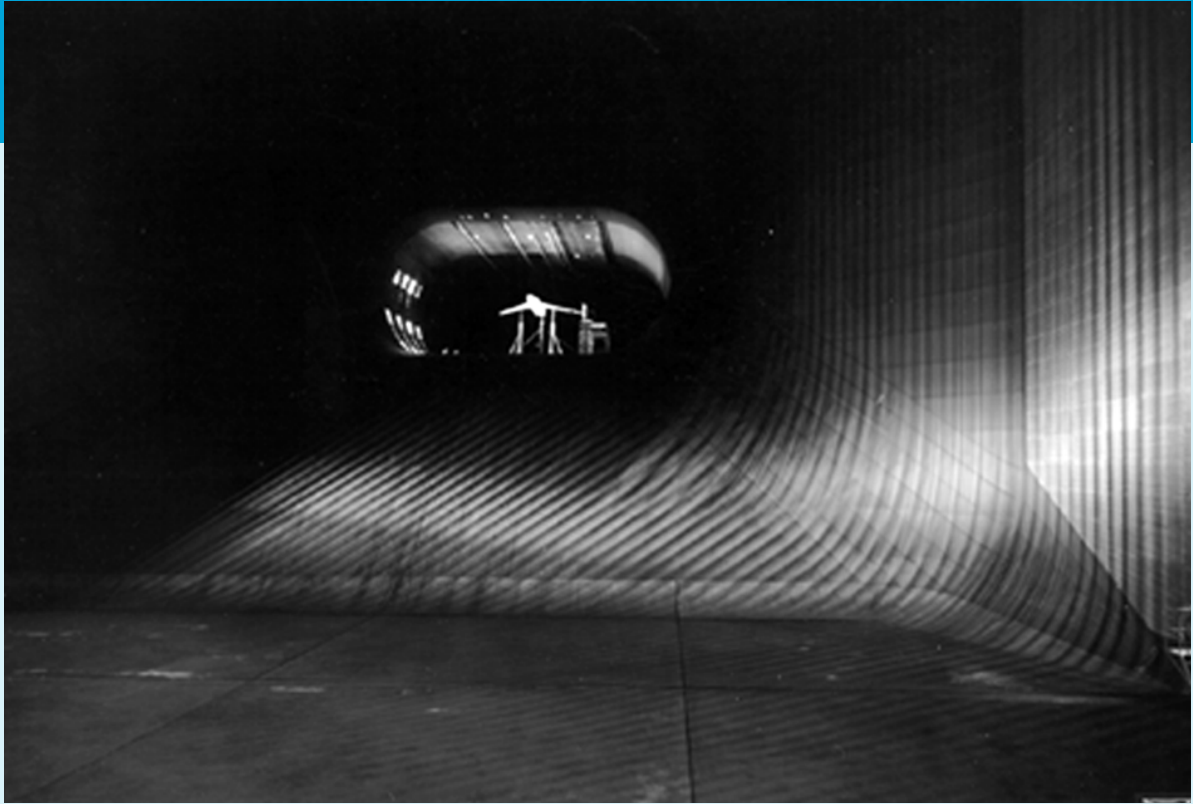
NACA's 40 x 80 foot wind tunnel at Ames Aeronautical Laboratory. The model shown here is 50 feet long.
