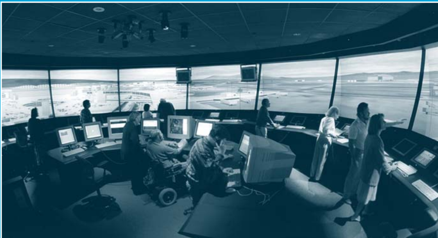
NASA “Future Flight Central,” the world’s first full-scale virtual airport control tower at Ames. The facility is designed to test ways to solve potential air and ground traffic problems at commercial airports under realistic airport conditions and configurations.
