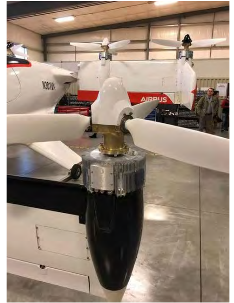
Variable pitch fan on Vahana aircraft (photo: Motivo)
