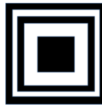
Figure 12: “Pickup” Area Marker (1m length square)
