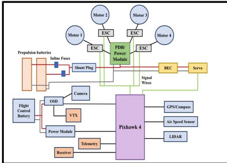
Figure 10: PDB/Power module diagram
