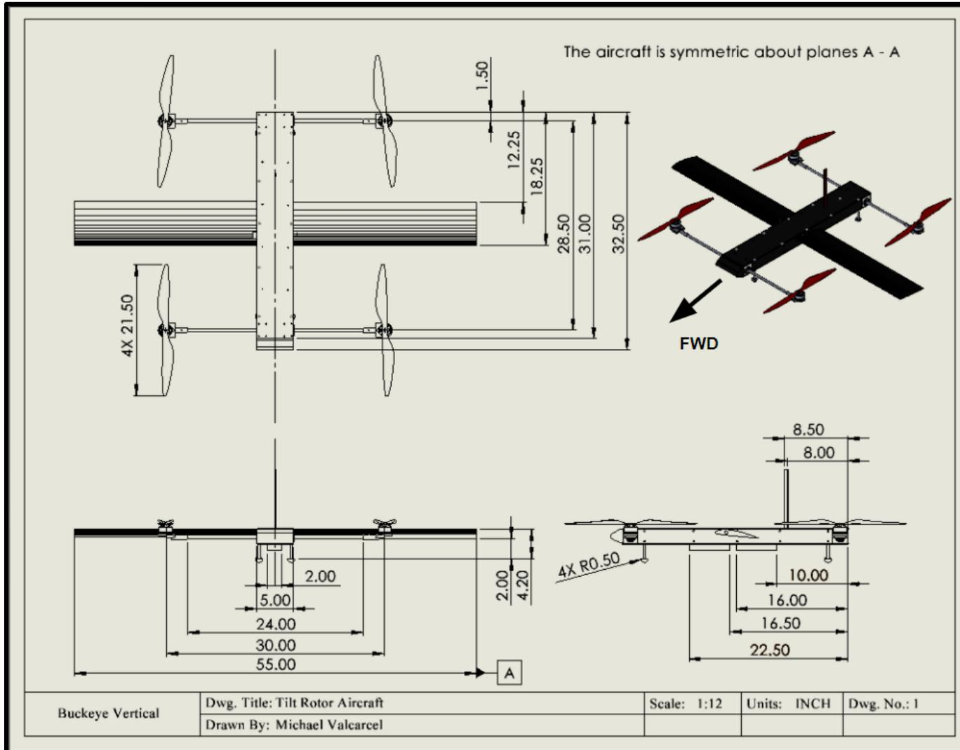
Figure 12: Engineering drawing of aircraft
