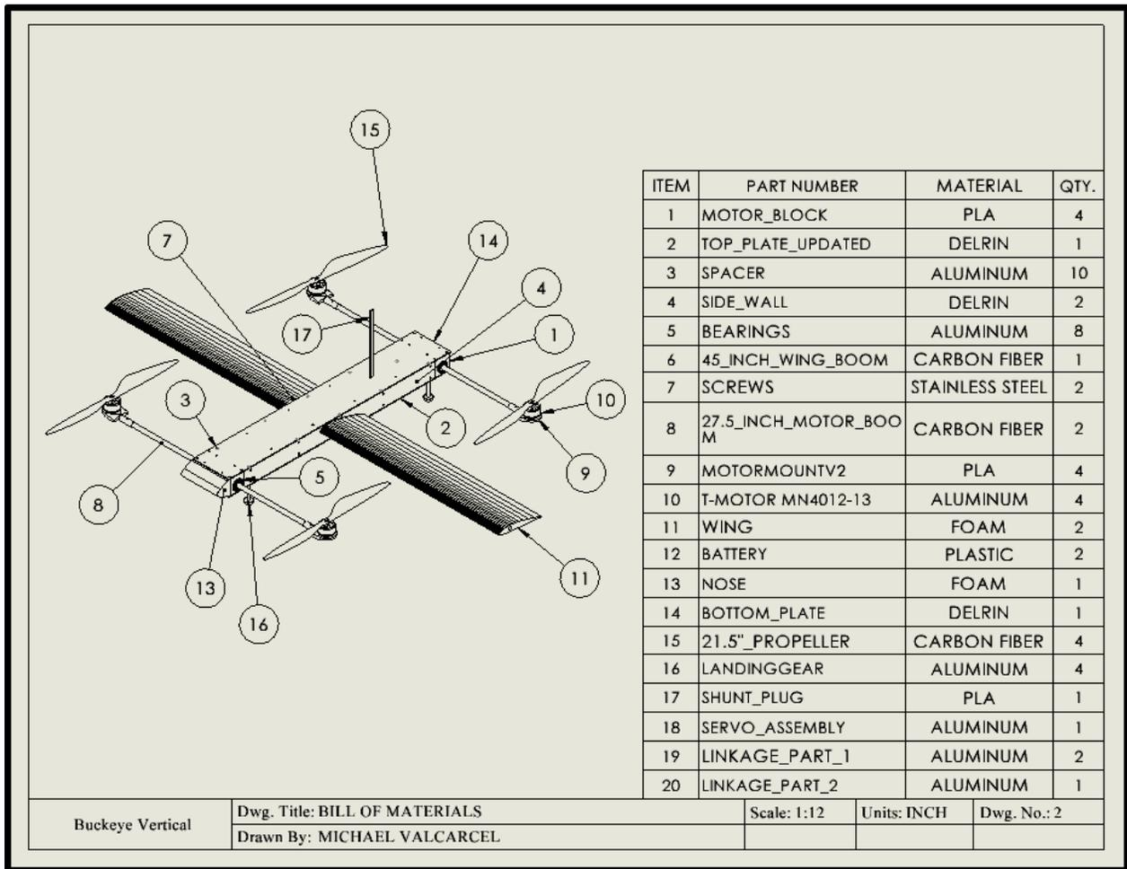
Figure 13: Engineering drawing of structural arrangements with bill of materials
