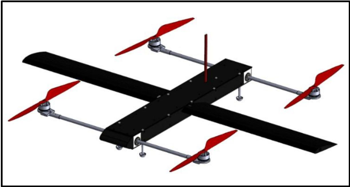
Figure 1: Isometric view of aircraft in vertical flight
