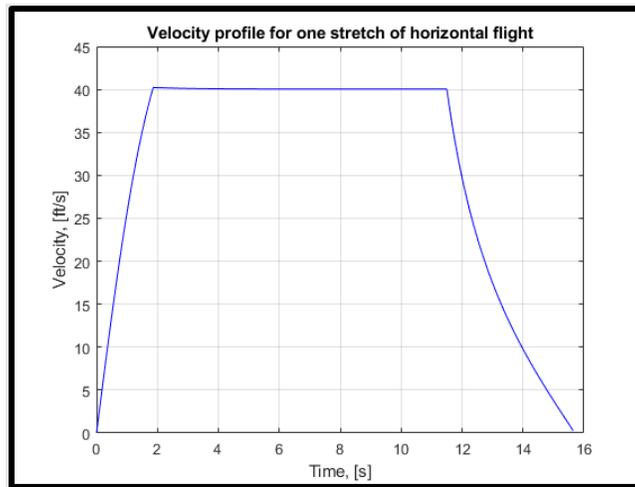
Figure 9: Velocity profile numerical solution for 500 ft stretch of straight flight
