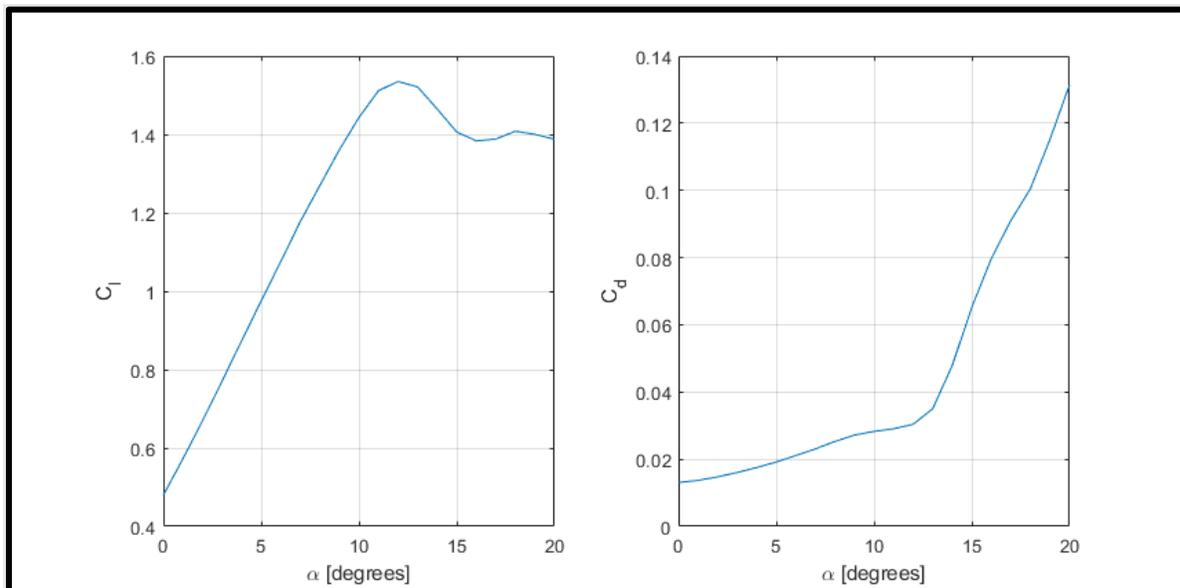
Figure 7: XFLR5 prediction of lift and drag variation with angle of attack for NACA 4313
