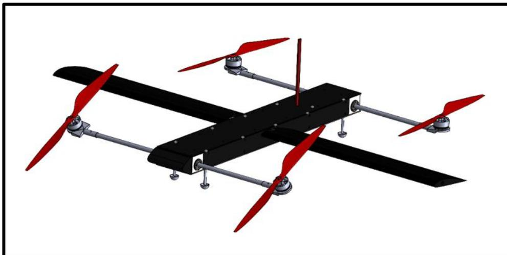
Figure 4: Isometric view of aircraft in forward flight
