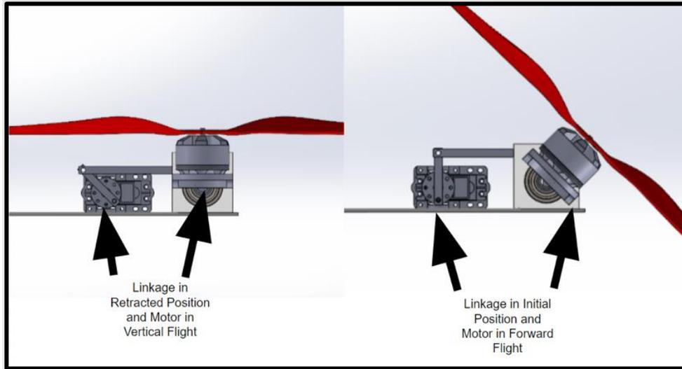
Figure 5: Tilt rotor with linkage assembly
