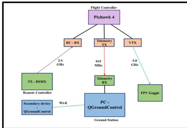
Figure 11: Pixhawk 4 flight controller diagram
