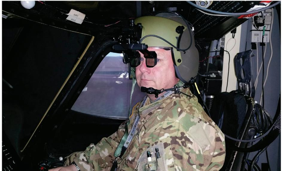
*Trials in the USAARL simulator will evaluate ICE-V symbology on both Panel Mounted Displays (PMDs) and head-tracked, binocular, wide-field-of-view Helmet Mounted Displays (HMDs). (USAARL)*
