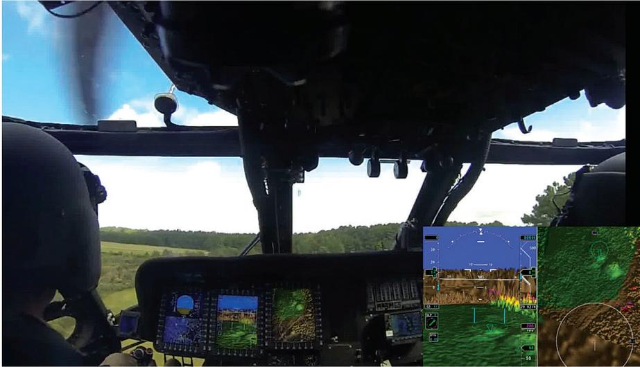
Honeywell Aerospace adapted its commercial Synthetic Vision Aviation Backbone (SVAB) to the DARPA Multi-Role, Multi-Function (MFRF) technology demonstration. (Honeywell)
