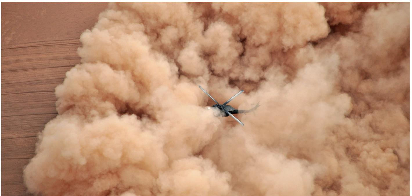
An AMRDEC UH-60 test aircraft generates a brownout dust cloud. The AMRDEC DVE-M program aims to mitigate brownout and other Degraded Visual Environments with integrated pilot cueing, advanced flight controls, and see-through sensors. (US Army Research Laboratory)
