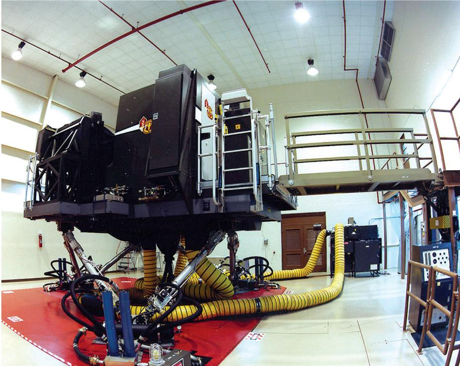
The US Army Aeromedical Research Laboratory has a UH-60 simulator able to collect crew biometrics in simulated Degraded Visual Environments. (USAARL)
