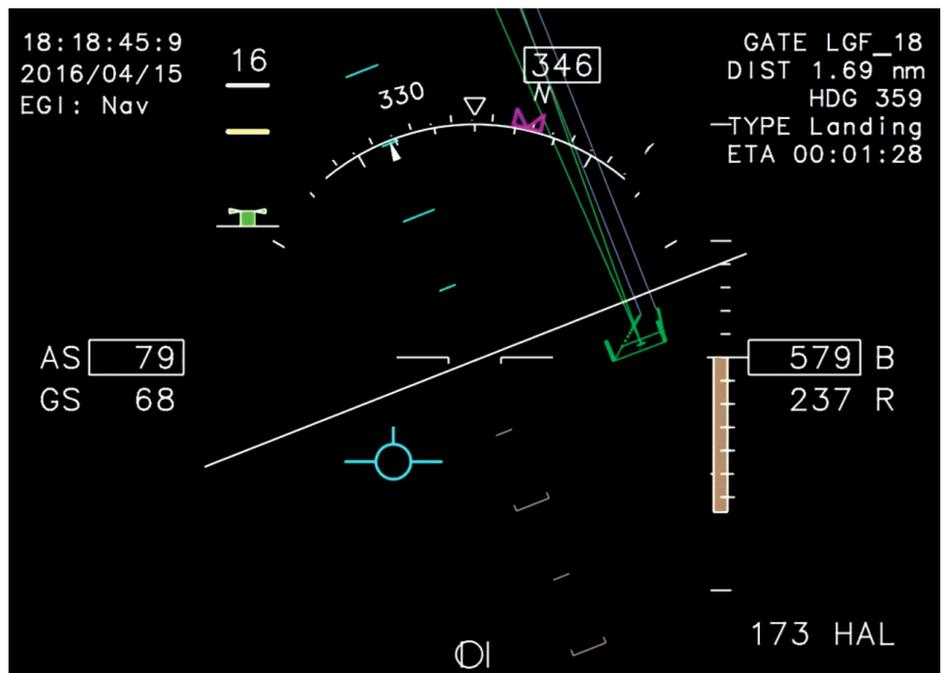
The USAARL simulator can display ICE-V symbology on Panel Mounted Displays. ICE-V symbology evolved from BOSS – the Brown-Out Symbology System -- and provides 2-D cues enroute and 3-D conformal symbology near the Landing Zone. (USAARL)
