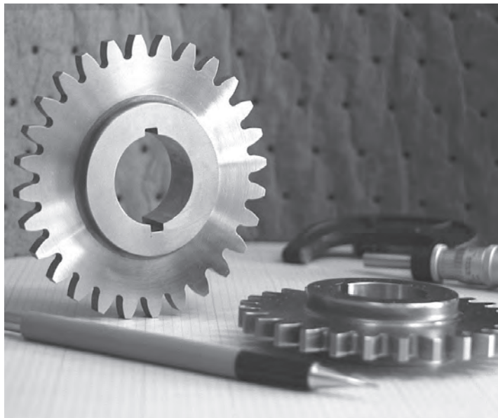
Sentient Science used NASA data generated by an aerospace-quality test gear to validate its DigitalClone wear predictions. (NASA)
