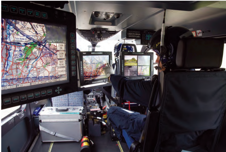
The London Police's Airbus EC145 twin-engine helicopters' video management systems (VMS) utilize a triple sensor camera system that feeds video into any of the five mission screens in the cabin. The police officer in the mid-cabin acts as the tactical commander.
