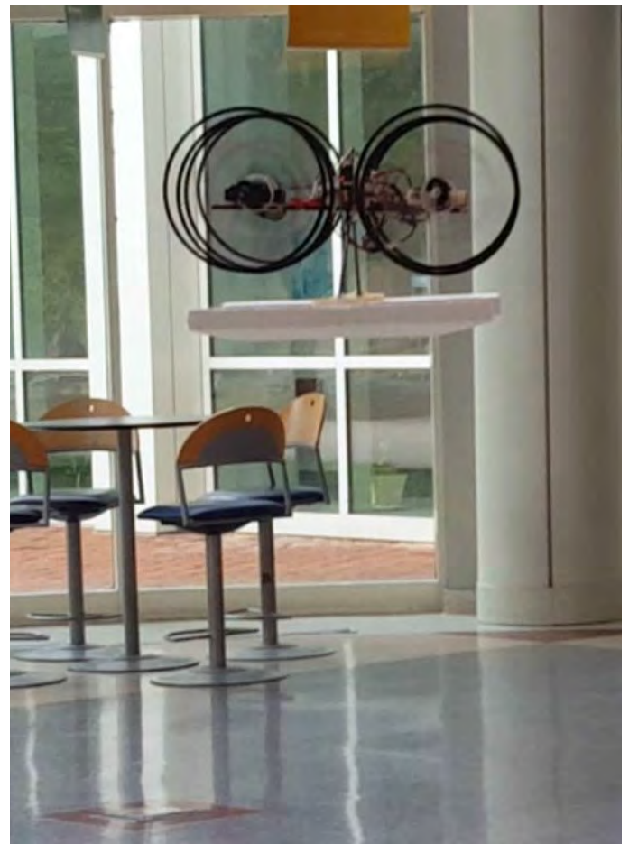
The multi-modal quadrotor cyclocopter can fly in the air and travel across the ground using its cyclocopter endplates as wheels. It is shown here with the foam pontoons for aquatic operations — the skids are raised for terrestrial locomotion. (Image via Elena Shrestha)
