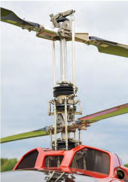
EDM sister company Dreiling Maschinenbau is building and testing the rotor systems. (EDM Aerotec photo)
