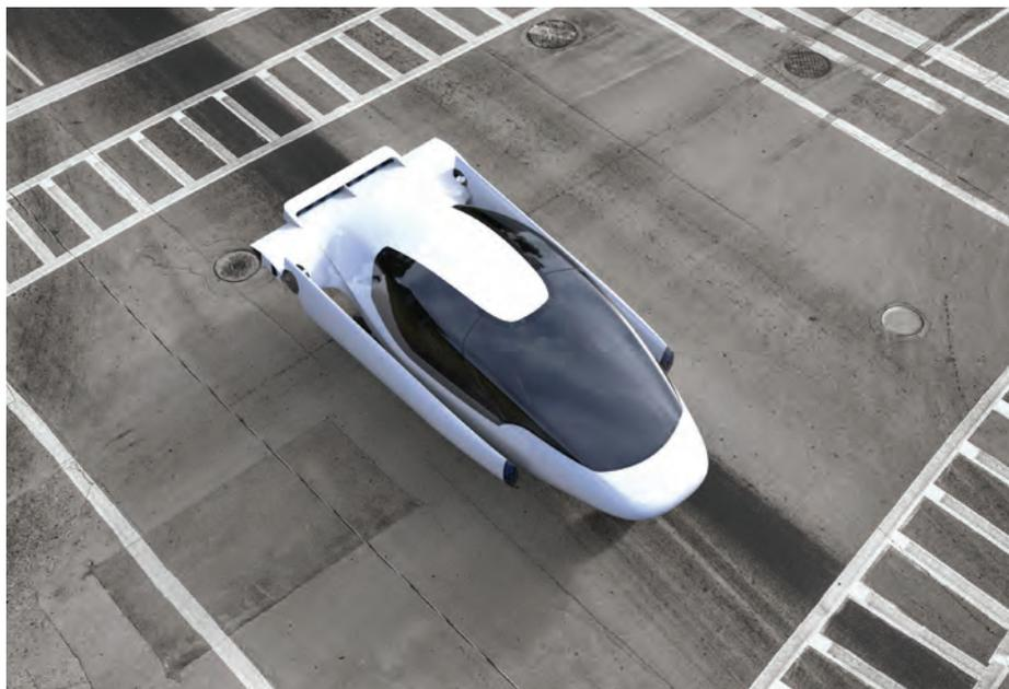
*Ilium Aviation is studying the feasibility of having a roadable capability; the canards retract into the fuselage and the wings could fold forward. (Ilium Aviation)*
