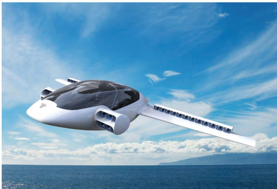
*The all-electric Ilium Jet uses 36 electric fans that tilt from vertical to horizontal. (Ilium Aviation)*
