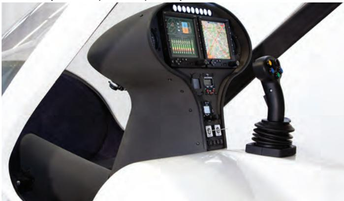
The e-volo VC200 uses 18 electric motors and a simple joystick for control. (e-volo photo)
