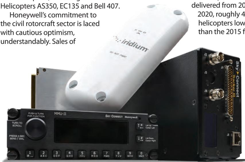
*Sky Connect Tracker III is a lightweight Iridium satellite transceiver enabling aircraft tracking and flight data monitoring. Combined with the optional Sky Connect MMU-II panel-mounted dialer, the system simultaneously supports two-way text messaging and voice telephony.*
