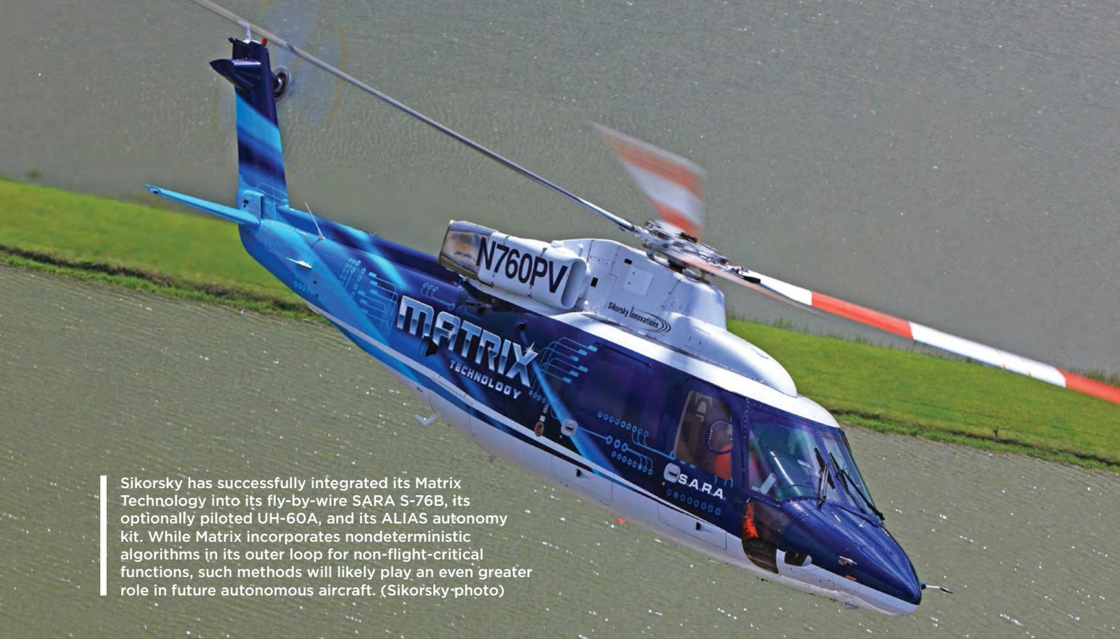
Sikorsky has successfully integrated its Matrix Technology into its fly-by-wire SARA S-76B, its optionally piloted UH-60A, and its ALIAS autonomy kit. While Matrix incorporates nondeterministic algorithms in its outer loop for non-flight-critical functions, such methods will likely play an even greater role in future autonomous aircraft. (Sikorsky-photo)
