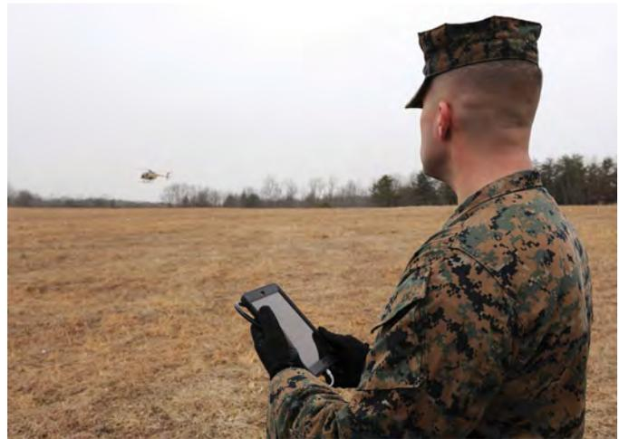
**An unskilled Marine operator directs an unmanned Boeing H-6U — equipped with the initial Autonomous Aerial Cargo/Utility System (AACUS) capability — from a tablet in April 2014. (Aurora photo)**
