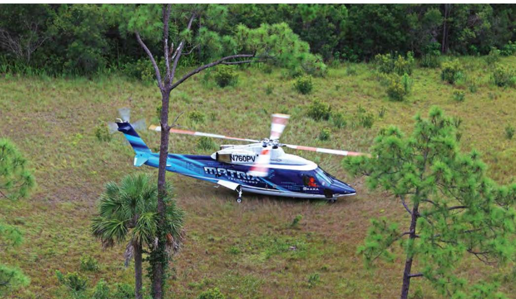
Sikorsky is looking at a variety of ways to incorporate autonomy into its current manned platforms. For example, in the event of an engine failure, a semi-autonomous helicopter could identify a suitable landing zone faster than a human pilot. Such image recognition capabilities leverage nondeterministic processes. SARA autonomously landed in a clearing in 2013. (Sikorsky photo)
