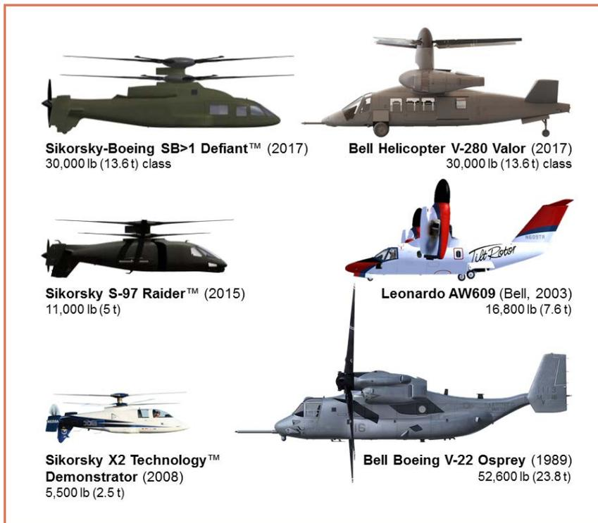
Shown above are provisional size comparisons of X2 and tiltrotor configurations, along with gross weight and first flight dates. (AHS International)
