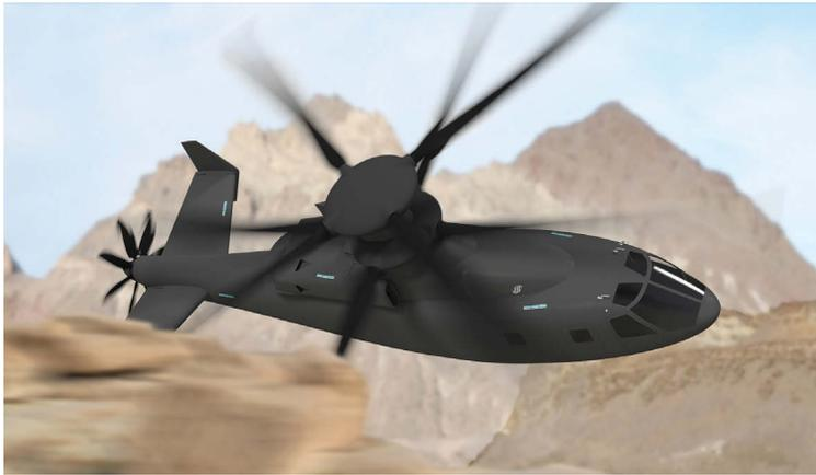
*The 30,000 lb (14 t) Defiant demonstrator is designed to satisfy key parameters in the JMR Mission Performance Specification aimed at a Future Vertical Lift — Medium. (Boeing graphic)*
