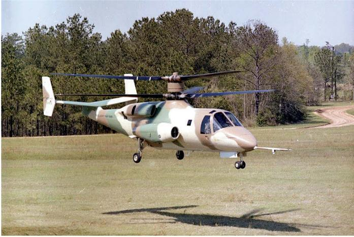
The Sikorsky X2-coaxial Advancing Blade Concept (ABC) was originally proven on the S-69/XH-59, flown between 1973 and 1981. It demonstrated 263 kt (487 km/hr) in a shallow dive. (US Army photo)
