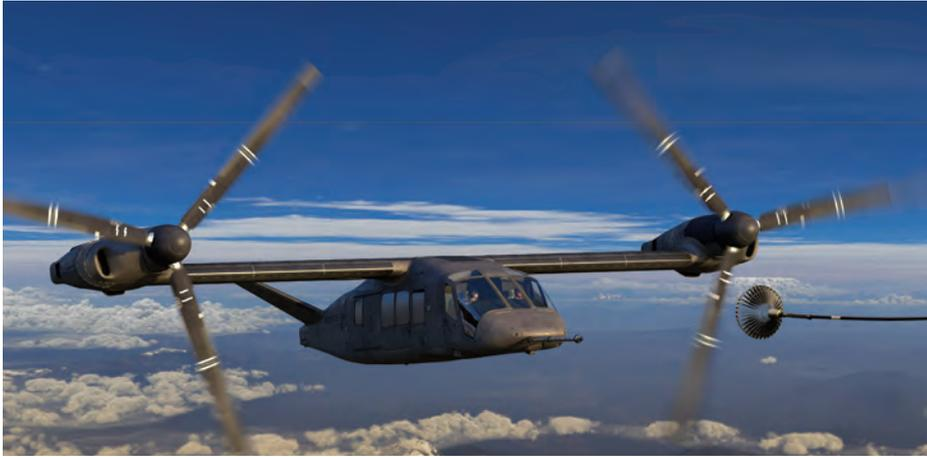
The larger ratio of proprotor diameter to fuselage weight results in Valor disk loading that is only two-thirds that of the V-22 Osprey. (Bell Helicopter)
