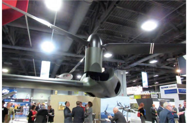
The latest V-280 mock-up shows the current configuration with a reduced-area V-tail and nacelle "cradle." (AHS International)
