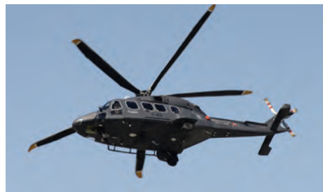
The AW149 was derived from the AW139 as a larger, military version. Although it has not yet found a military customer, the civil version — the AW189 — has been a runaway success.
