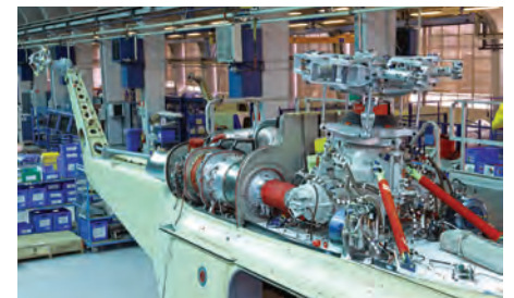
Vergiate integrates the British transmission and Canadian engines with the fuselage, rotor hubs, blades, avionics, etc., from other AgustaWestland plants around Italy.
