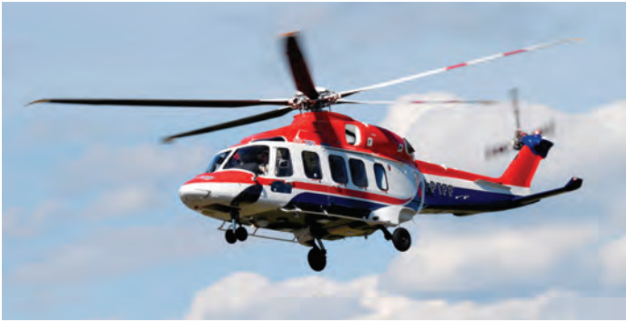
The AW189 is considered a “super medium” aircraft. Like the AW139, its main gearbox benefits from an unsurpassed 50 minute “dry-run” capability.
