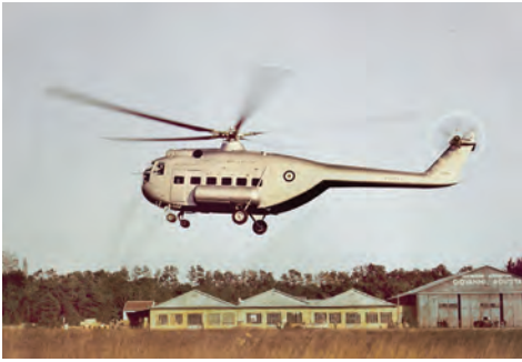
The three-engine 13 t (28,400 lb) A.101G was Agusta's first indigenous design. It first flew in October 1964, but was dropped in 1971.
