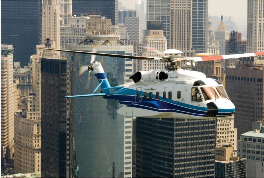
Commercial helicopters like the S-92 operating over noisy Manhattan must still adhere to Fly Neighborly procedures including defined noise avoidance routes. Current noise models do not take into account 'urban canyon' acoustics. (Sikorsky Aircraft)
