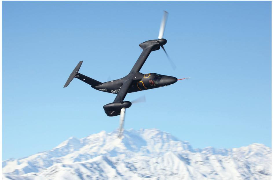
*With proprotors in airplane mode, the AW609 tilt rotor avoids the high-amplitude, low-frequency noise associated with a helicopter. Helicopter-like landings nevertheless put the revolutionary rotorcraft back in noise-sensitive environments. (AgustaWestland)*
