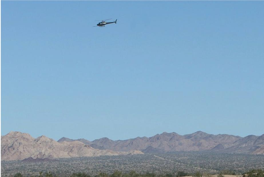
*Acoustic measurements were made with a light civil AS350B (shown at Salton Sea) and a medium military EH-60L helicopter at three different elevations with the same pilots flying identical profiles. (NASA photo)*
