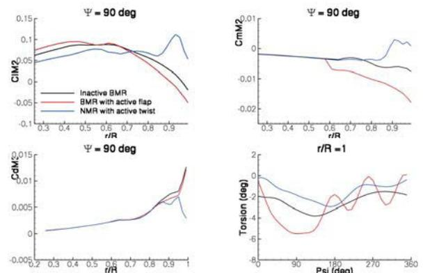
Figure 16: Effect of active flap (BMR) and active twist (NMR) laws on the aerodynamic coefficients ( $\psi = 90^\circ$ ) and on the torsion deformation ( $r/R = 1$ ) -  $C_T/\sigma = 0.06$ ,  $V_h = 130$  kts
