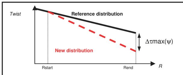
Figure 1: Scheme of the active twist deflection model
