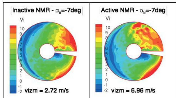
Figure 9: Distribution of the induced velocity fields for the inactive NMR (left), and the NMR with active twist (right) -  $\alpha_d=-7^\circ$
