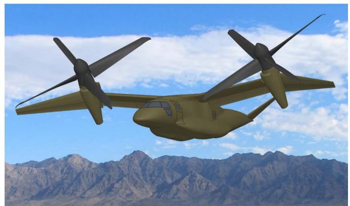
Karem's FVL Capability Set 3-compliant configuration is the KVL-3 Mustang. Karem hopes to run a full-scale powered single-rotor tiedown test, in both helicopter and propeller modes, as part of JMR. (Karem Aircraft graphic)
