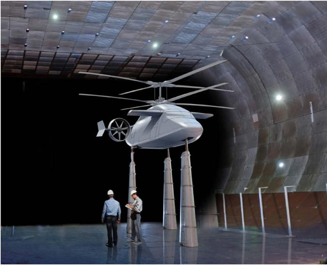
AVX hopes to test a half-scale Coaxial Compound Helicopter in the NASA 40 ft by 80 ft wind tunnel testing as part of an extended JMR Technology Investment Agreement. Like Bell's V-280, the CCH attack and utility variants have common fuselages. (AVX Aircraft graphic)
