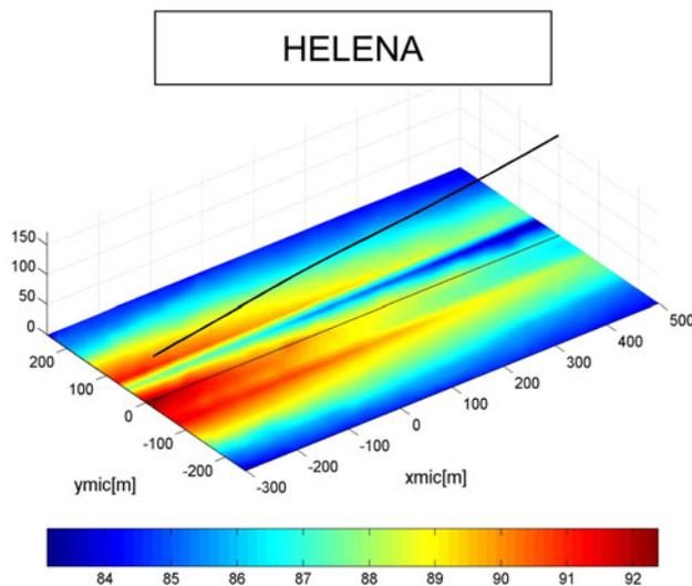
**Fig. 10** On ground noise impact of approaching helicopter: HEL-ENA computation (copyright Eurocopter)
