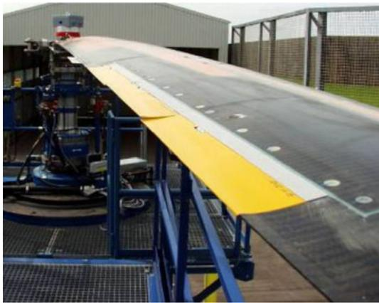
**Fig. 13** Blade with active flaps ‘blue pulse’ (copyright Eurocopter)
