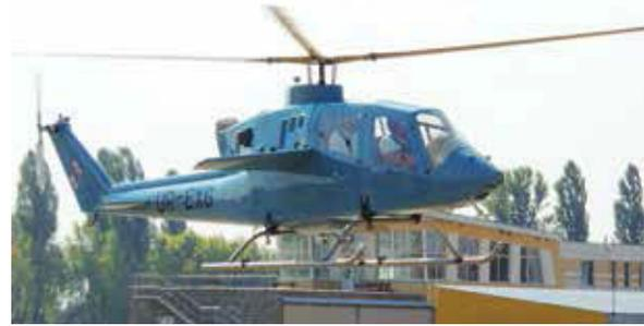
The Softex Aero VV-2 in flight. The tandem-seat aircraft is available as a kit, as an attack helicopter and/or unmanned. (Photo courtesy of Viktor Vashchenko)
