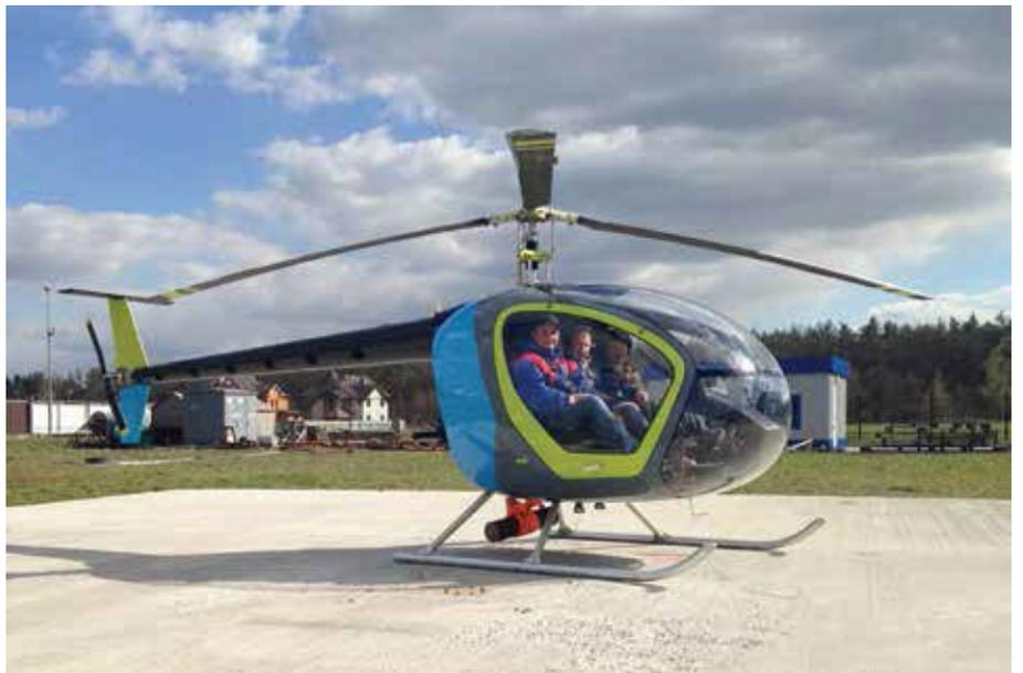
The Scout has three-abreast seating and is now being prepared for sale in the US. (Photo courtesy of Scout Aero, LLC)
