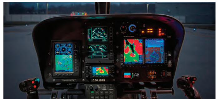
In 2012, Kitchener Aero Avionics receive a supplemental type certificate (STC) to install the Garmin G500H glass cockpit in the single-engine Airbus EC120 Colibri. (Kitchener photo)
