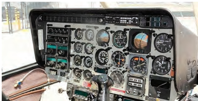
The Bell 206 was approved for IFR operations in the 1990s with an instrument panel that today looks rather primitive. (Photo via Paul Schaaf)
