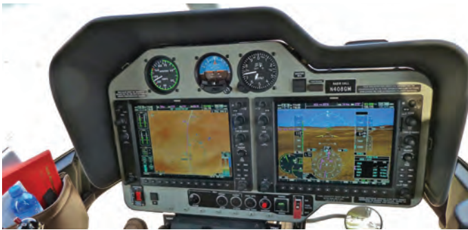
The Bell 407G-series of single-engine helicopters feature the Garmin G1000H. Bell introduced the glass cockpit to increase the amount of useful information presented and to improve the pilot's situational awareness. (407GX cockpit photo courtesy of George Mandes)
