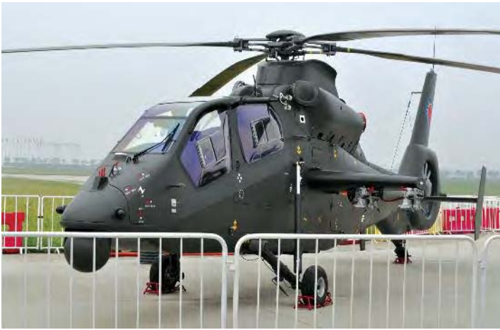
The Avicopter Z-19 scout/attack helicopter is a distant derivative of the Dauphin.
