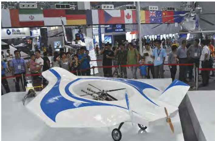
The Feihong is a coaxial ducted rotor aircraft that Avicopter says it has tested extensively. (The AC352 and AC311 can be seen in the background.)
