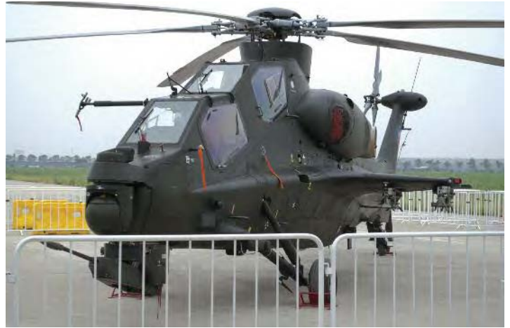
The indigenous Z-10 is a 7 ton attack helicopter built by Avicopter subsidiary Changhe Aircraft Industries Corporation.
