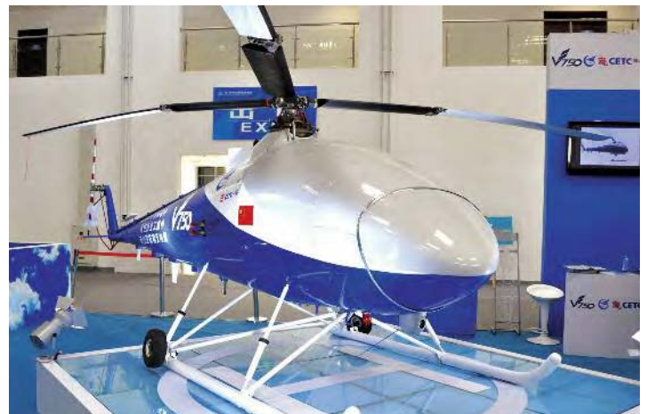
The Freesky-AVIC-CETC V750, derived from the Brantly B-2B, is the largest unmanned rotorcraft to have flown in China.
