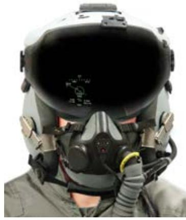
The Joint Helmet Mounted Cueing System (JHMCS) puts targeting symbology into fighter pilot helmets with a narrow field of view. It is meant to cue missile seekers to off-axis targets in air-to-air combat. (Rockwell Collins)
