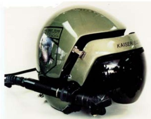
The Comanche Helmet Integrated Display Sighting System (HIDSS) started with the Kaiser Electronics Wide-Eye helmet display to provide a wide field, biocular field of view with overlap. (Rockwell Collins)
