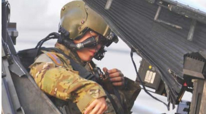
The Apache Integrated Helmet And Display Sighting System (IHADSS) uses a monocular head display unit to show imagery from the AH-64 modernized night pilotage sensor and modernized target acquisition and designation sight. (US Army)
