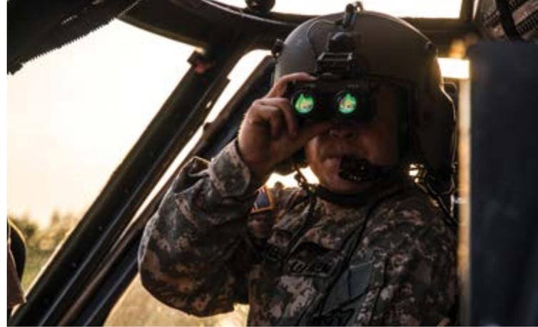
A medevac Black Hawk pilot adjusts night vision goggles. ANVIS HUDs such as the Elbit HDTs show flight symbology on a day or night monocular within the 40-degree field of view of NVGs. (US DOD)
