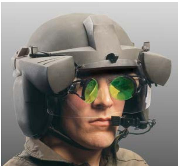
The Comanche HIDSS ultimately had two AMLCD monoculars overlapped for a 52-by-30-degree field of view. (Rockwell Collins)
