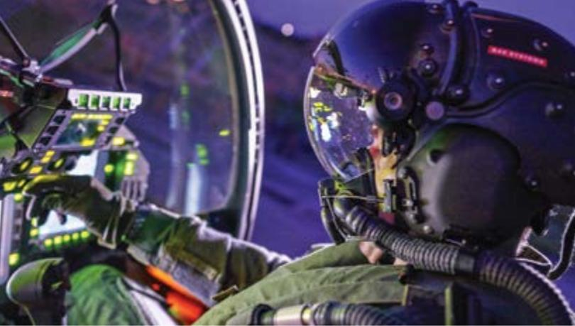
The BAE Striker II system used in Gripen and Typhoon fighters has a wide-field-of-view visor display with color symbology and co-picture-in-a-picture capability for situational awareness. (BAE Systems)
