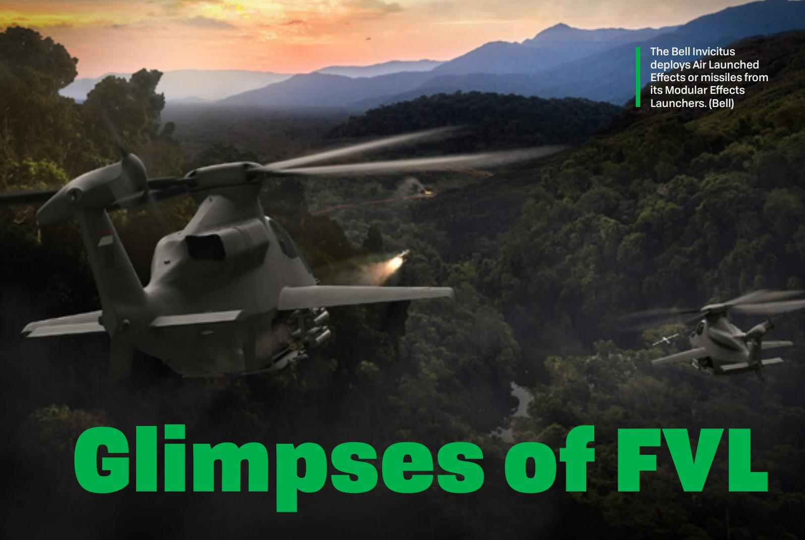
The Bell Invictus deploys Air Launched Effects or missiles from its Modular Effects Launchers. (Bell)
