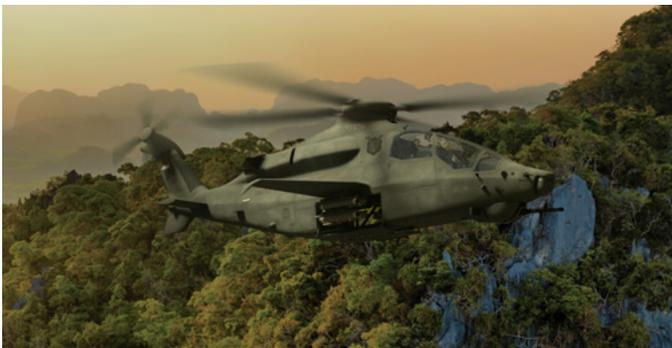
The Bell Model 360 Invictus stows its modular effects launchers in under-wing bays to deploy ALE or kinetic weapons. (Bell)
