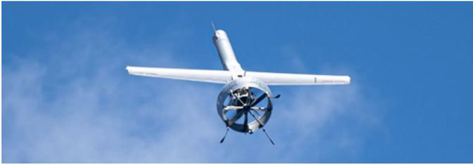
The Martin V-BAT UAS was one of the runway-independent unmanned aircraft systems tested by the Army to make an informed choice on the Future Tactical UAS. (US Army)
