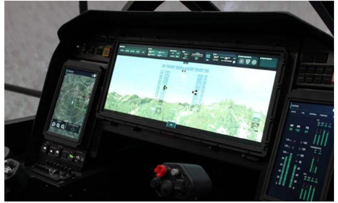
One concept for the Bell 360 FARA cockpit centers on a large touch-screen to manage sensor imagery and systems information. (Bell)
