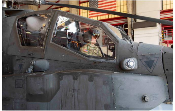
A wide field-of-view, color, helmet-mounted display tested in an Apache attack helicopter could also be used in FARA and FLRAA cockpits. (US Army)
