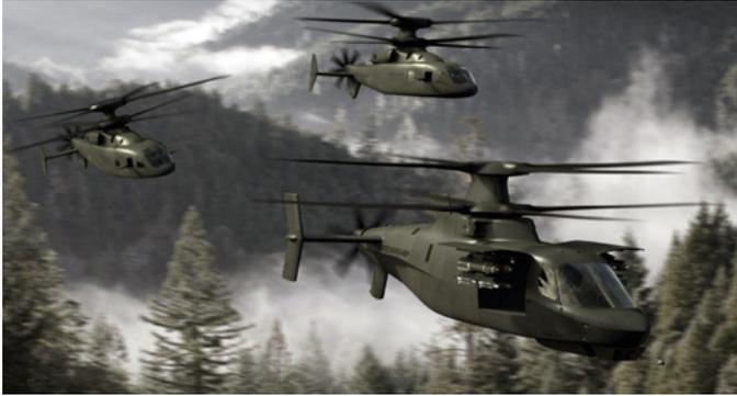
Sikorsky's S-103 Raider X for (foreground) is based on the test data and lessons learned from its S-97 Raider, as well as the Sikorsky-Boeing SB>1 Defiant (shown in the rear) development work for JMR/FLRAA. (Sikorsky)
