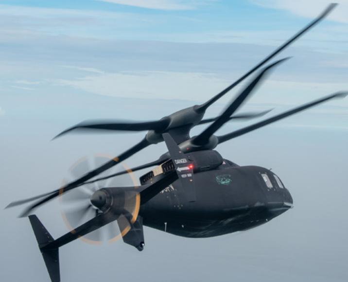
The Sikorsky-Boeing SB>1 Defiant continues its Joint Multi-Role flight test program to provide data for a Future Long Range Assault Aircraft. (Sikorsky)
