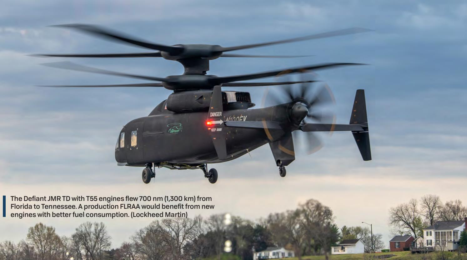
The Defiant JMR TD with T55 engines flew 700 nm (1,300 km) from Florida to Tennessee. A production FLRAA would benefit from new engines with better fuel consumption. (Lockheed Martin)
