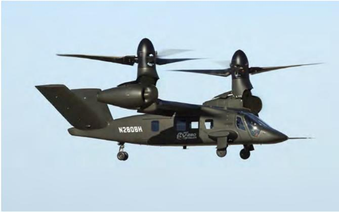
The Bell V-280 Valor JMR TD models an advanced tiltrotor FLRAA with fixed engines for greater reliability and maintainability. (Bell)
