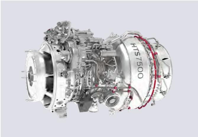
The Honeywell HTS7500 leverages its T55 lineage and commercial engine technologies to give the Defiant X an on-condition engine for FLRAA requirements. (Honeywell)
