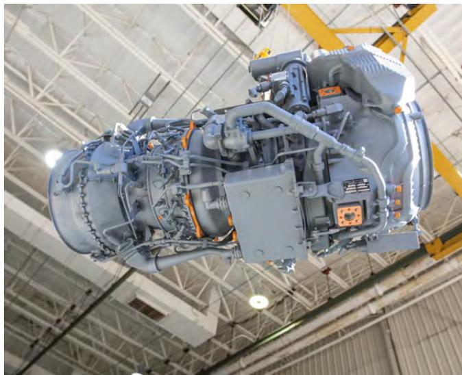
A 3D-printed full-scale model of the GE T901 engine hangs from a sling in the Boeing Mesa facility during a mock-up fit check in an Apache helicopter. (Boeing)
