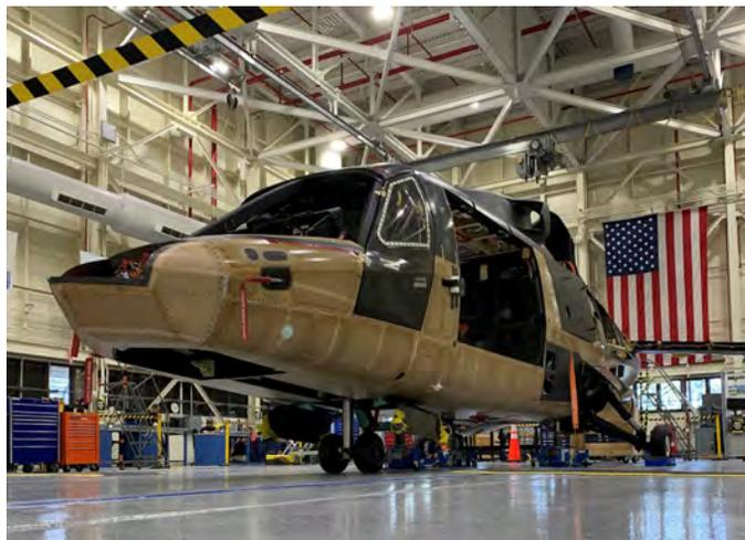
The Sikorsky Defiant X FARA competitive prototype is in assembly at West Palm Beach, Florida, and will fly with the Army’s T901 improved turbine engine. (Lockheed Martin)
