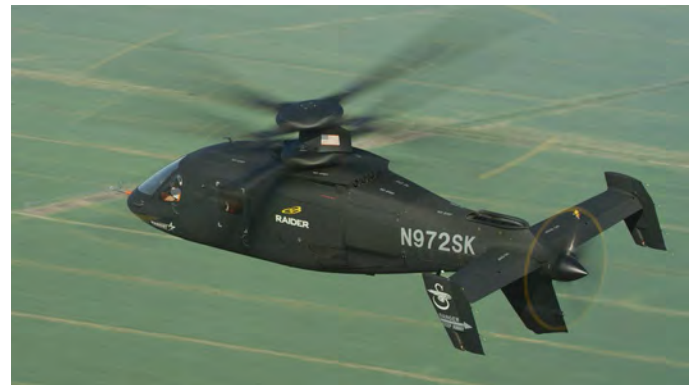
The 11,000 lb (5 t) Sikorsky Raider demonstrator has been flown to to 200 kt (370 km/h) and is a risk-reduction demonstrator for both the larger FARA (CapSet 1) and Defiant/FLRAA (CapSet 3) programs. (Sikorsky photo)
