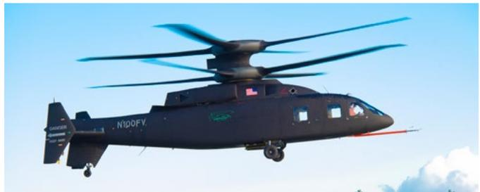
As of press time, the SB1 had been flown at 20 kt (37 km/h) in every direction, including hover-out-of-ground-effect (HOGE). (Sikorsky-Boeing photo)
