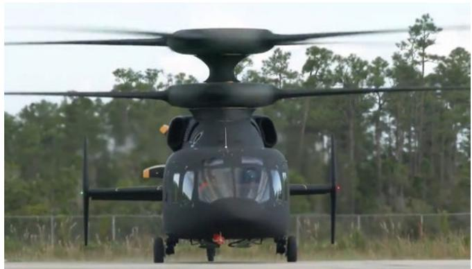
The Sikorsky-Boeing team added the rotor fairings after to its fourth flight, which was made on Sept. 24. (Image from Sikorsky-Boeing video)
