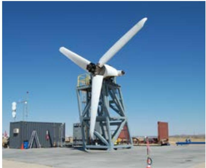
**Karem's 36-ft diameter, single-rotor tiedown testing is now underway to demonstrate the company's suite of optimum speed tiltrotor (OSTR) technologies. (Karem photo)**
