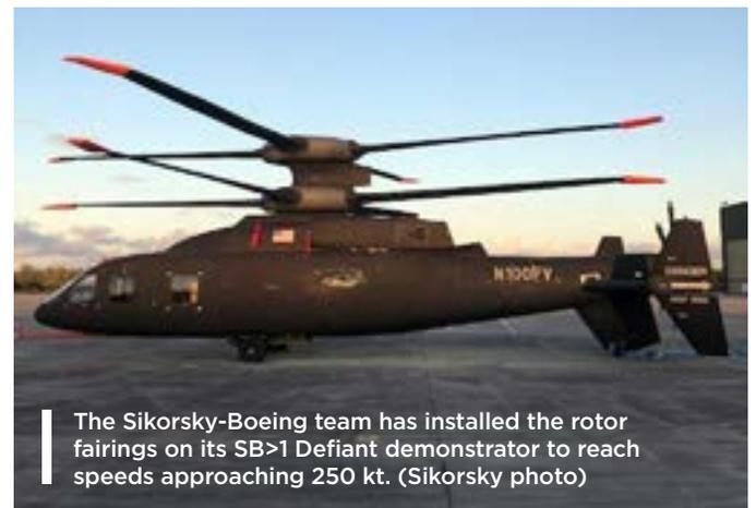
The Sikorsky-Boeing team has installed the rotor fairings on its SB-1 Defiant demonstrator to reach speeds approaching 250 kt. (Sikorsky photo)
