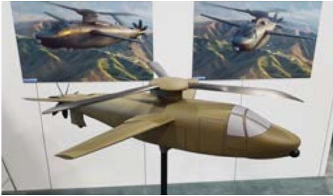
Karem's AR40 active-rotor, winged compound design for FARA features a swiveling tail rotor thruster for both anti-torque and high-speed flight. (VFS staff photo)
