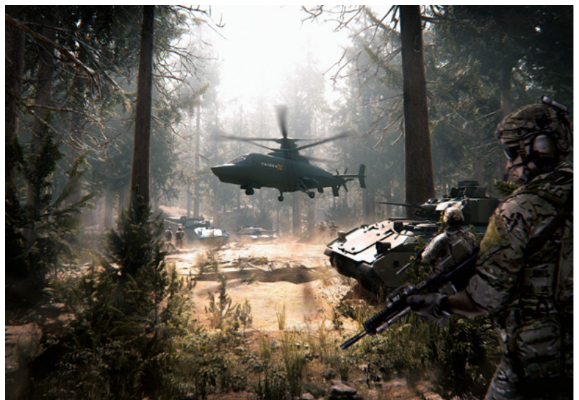
The FARA gross weight limit of 14,000 lb (6.4 t) makes Sikorsky’s Raider X concept nearly 25% heavier than its S-97 Raider demonstrator. (Sikorsky)
