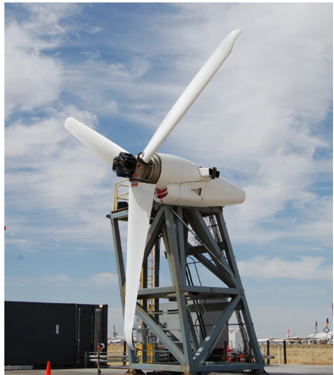
Karem is conducting high-speed tiedown tests of its 36-ft (11-m) diameter OSTR rotor.
