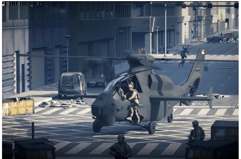
The Army limited FARA to a 40-ft (12-m) rotor diameter to allow operations in urban canyons, such as shown here with the Bell 360 Invictus. (Bell)
