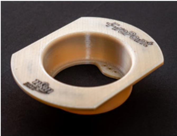
The US Army Aviation and Missile Command has begun qualifying 3D printed aircraft parts like this wire bundle grommet. (US Army)
