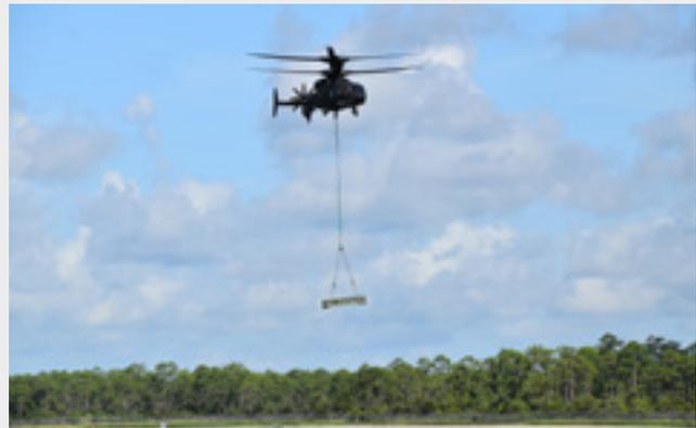
Sikorsky and Boeing made the main gearbox of the SB>1 Defiant 25% lighter than historical projections, using advanced materials and 3D modeling. Here it demonstrates its external lift capability. (Sikorsky)
