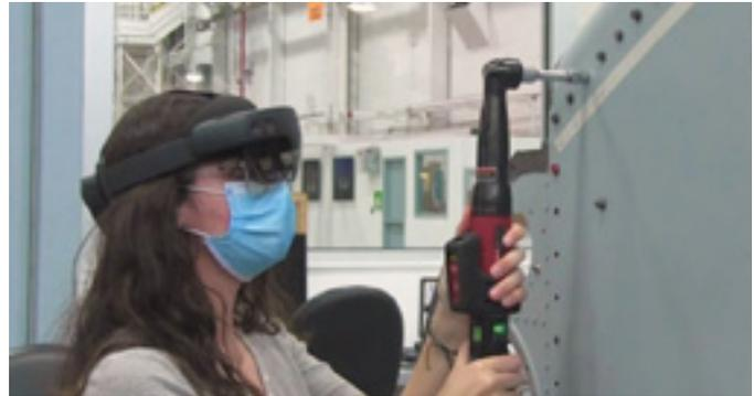
Sikorsky extends the digital thread to the manufacturing floor with digitally-enabled torque wrenches and glasses that show workers when nuts are torqued properly. (Sikorsky)
