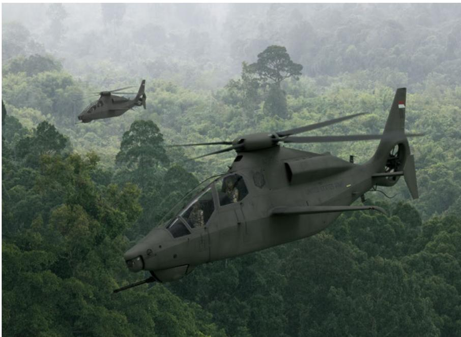
The Bell Model 360 Invictus is one approach to FARA and uses a fixed wing to attain higher speed and greater range than legacy helicopters. (Bell)
