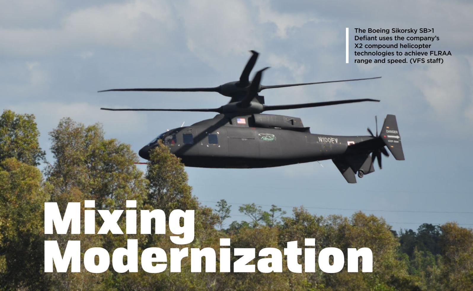
The Boeing Sikorsky SB>1 Defiant uses the company's X2 compound helicopter technologies to achieve FLRAA range and speed. (VFS staff)
