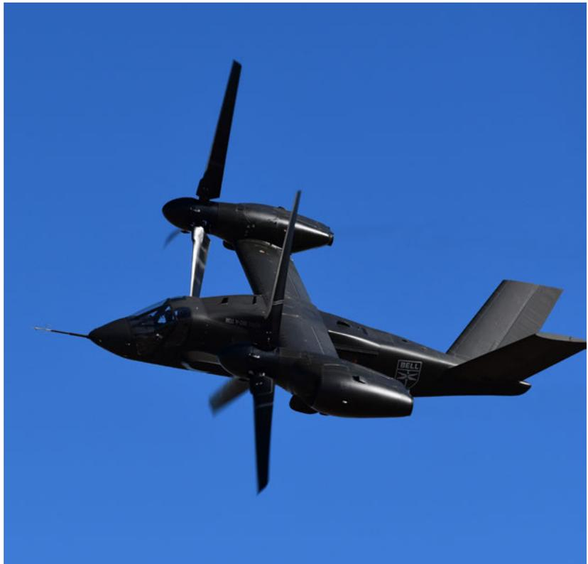
The Bell V-280 Valor JMR technology demonstrator offers a tiltrotor path to a program of record for a Future Long Range Assault Aircraft. (VFS staff)
