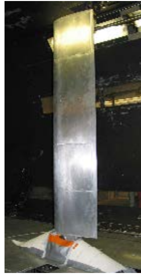
Full-sized Heliplane test hardware included a rotor blade aerodynamic test article.
