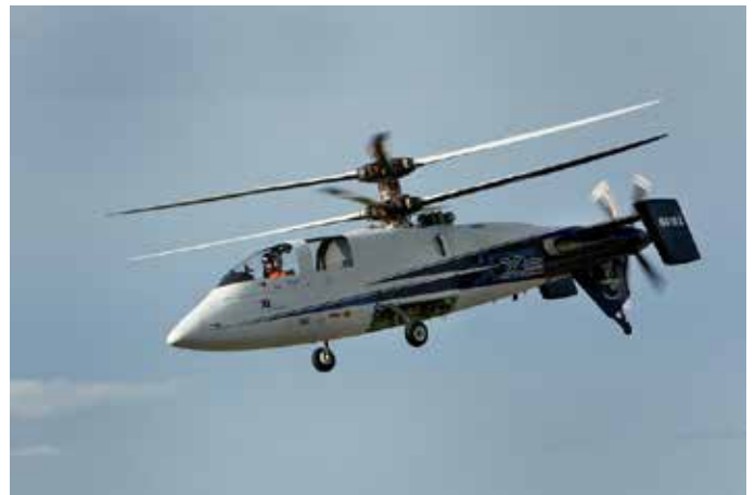
Sikorsky's X2 demonstrator integrated a coaxial lift-offset rotor, a pusher propeller and other new technologies for the first Sikorsky Innovations pillar — speed.
