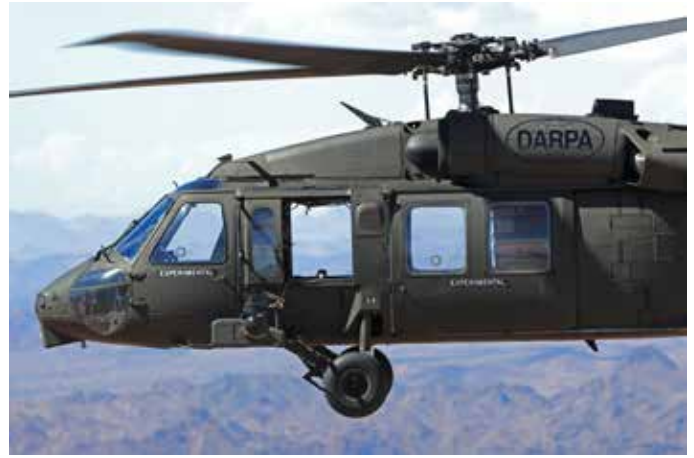
DARPA-sponsored autonomy development enabled an uncrewed Black Hawk to fly tactical missions.
