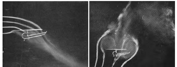
Jan Meijer Drees published wind tunnel test photos using smoke to study helicopter rotor flow. (NLR photos via Gordon Leishman)
