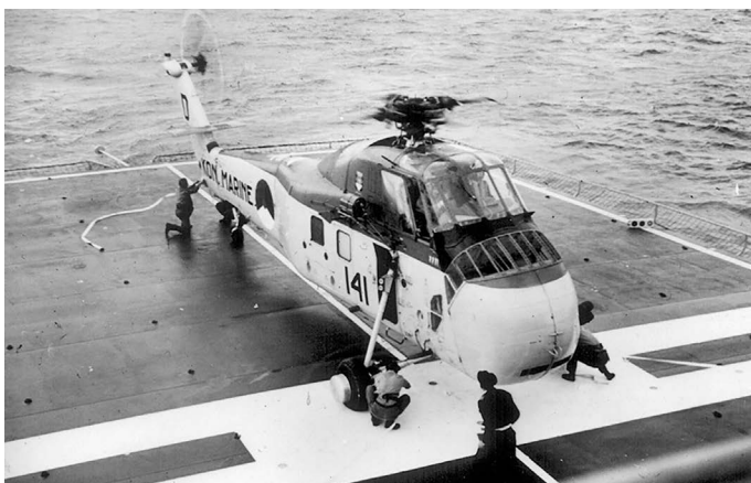
The HNLMS Poolster, the first Dutch navy ship equipped with a helicopter flight deck and a hangar made its maiden voyage in 1963. This photo is of the Sikorsky S-58 Seabat shipborne trials the following year. (NLR photo)
