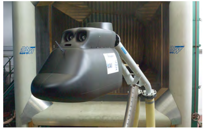
NLR designed and manufactured air intake models for the KAI Surion. This one was tested in the German-Dutch Wind Tunnels' (DNW) Low-Speed Wind Tunnel in Braunschweig, Germany (NWB). (NLR photo)
