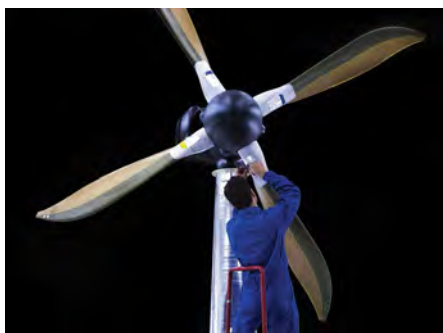
A half-model tiltrotor test at DNW in Marknesse in 2007 as part of the TILTAERO program. (DNW photo)
