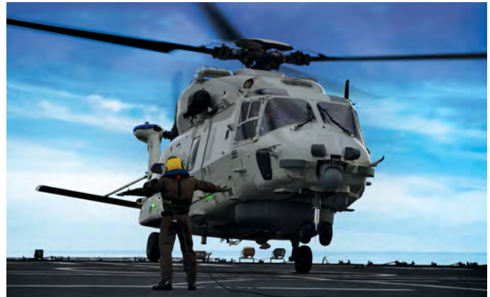
NLR was a key player in the development of the NH90, including support for shipborne testing, such as these sea trials with the NH90 NFH onboard a RNLN ship in 2011. (NLR photo)
