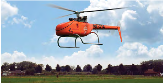
NLR is converting this Geocopter GC-201 drone to electrical power. (NLR photo)
