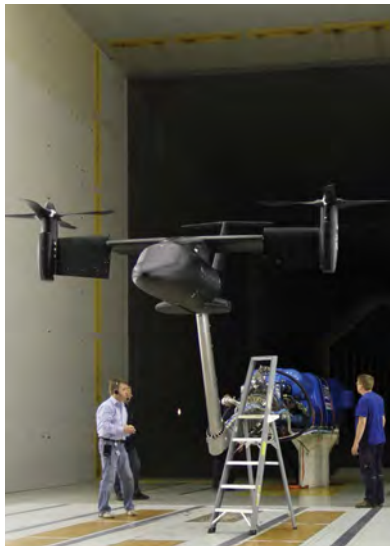
As part of Clean Sky, NLR is supporting tiltrotor research, including this 2013 testing of the AgustaWestland ERICA configuration in the DNW Large Low-Speed Facility (LLF) in Marknesse, The Netherlands. (DNW photo)
