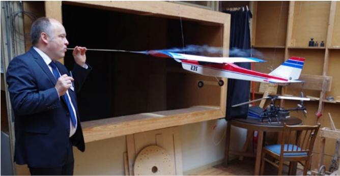
Dr. Steffen demonstrated flow visualization of a model in the Focke Wind Tunnel.
